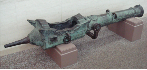
Fig. 5: The most common Folangji gun was the Portuguese berço , a breech-loading swivel gun. Source: https://commons.wikimedia.org/wiki/File:Oda_Nobunaga_swivel_breech_loading_gun.jpg
